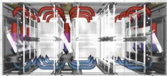
Top view – air flow detail – closed air-loop architecture with side coolers
