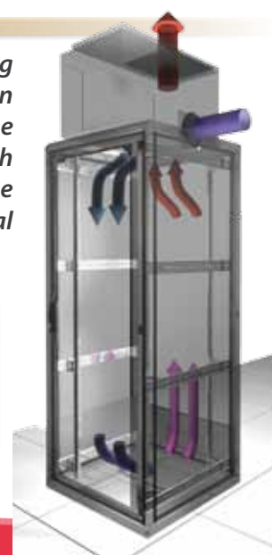
Air flow through the rack – top mount cooling
